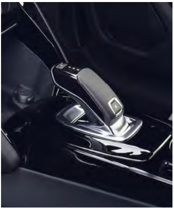
Electric Impulse Automatic Gearbox Control
